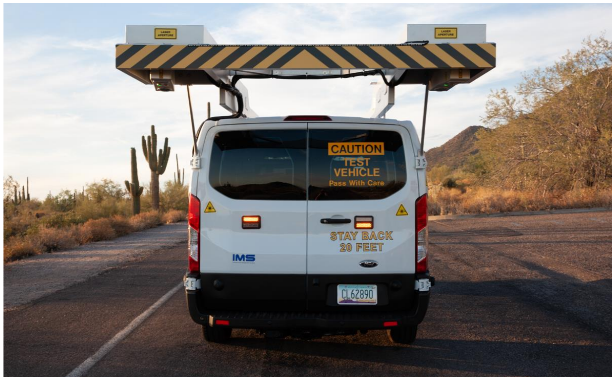
Figure 10 - LCMS2 data collection vehicle
