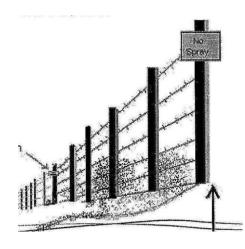
You will need to install (2) two signs. The signs should be white with black lettering, 12"x18". The signs must be clearly visible and placed on the right-of-way line. Failure to maintain signage may result in inadvertent application of herbicides.
