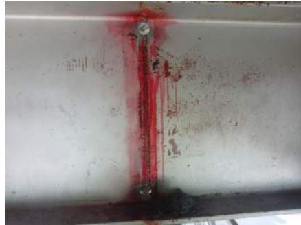
Cracked Splice on Girder 3 in Span 4 West Splice (Testing and Crack Tips)
